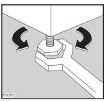
Any necessary adjustment can be made with a spanner. Accurate levelling prevents vibration, noise and displacement of the machine during operation. Never place cardboard, wood or similar materials under the machine to compensate for any unevenness in the floor.
